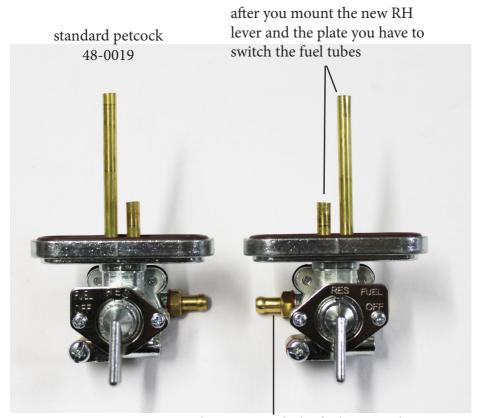
you have to switch the fuel pipe outlet to the other side
