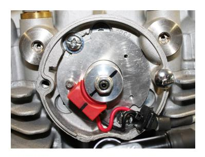
Reinstall the gas tank and proceed as follows to set the timing. A strobe type timing light is required to set the timing.
